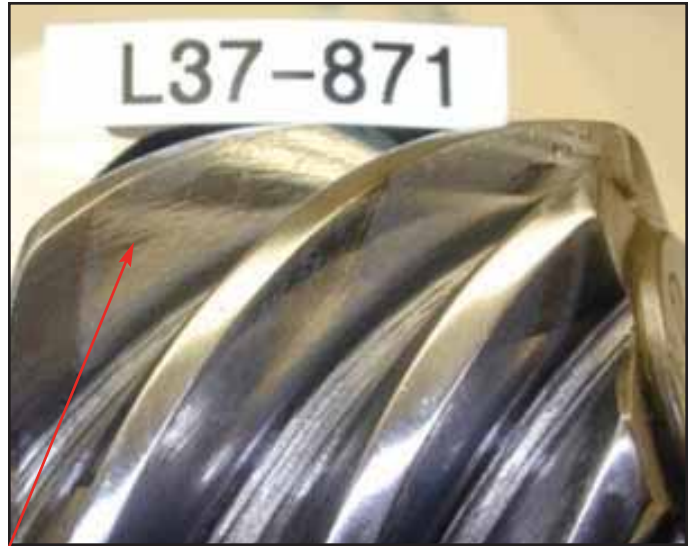
Pinion gear - original machine marks still present.
