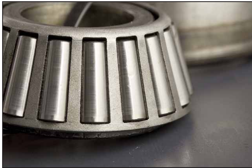
Pinion tapered roller bearing in like-new condition.
