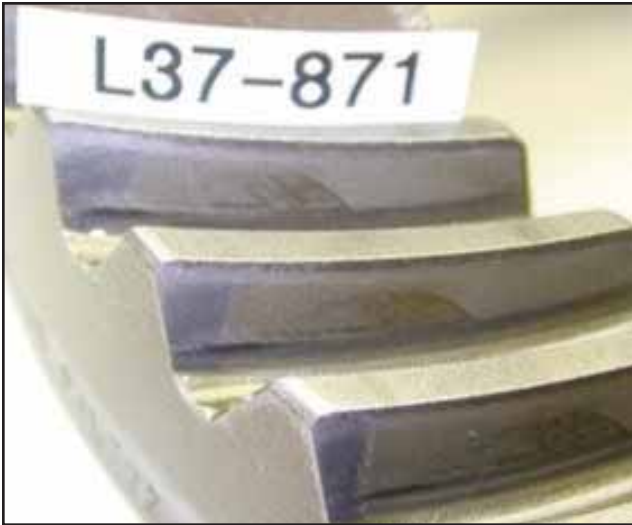
Ring gear exhibits very low wear.
